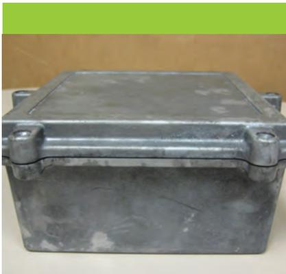
Figure 1. Aluminum housing used in testing.
