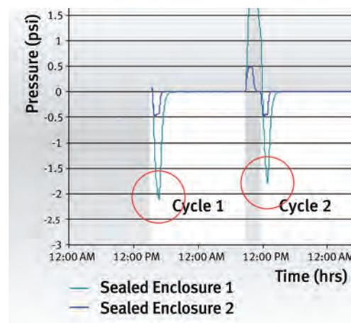
Figure 6. Pressure differentials for first sealed enclosure.
