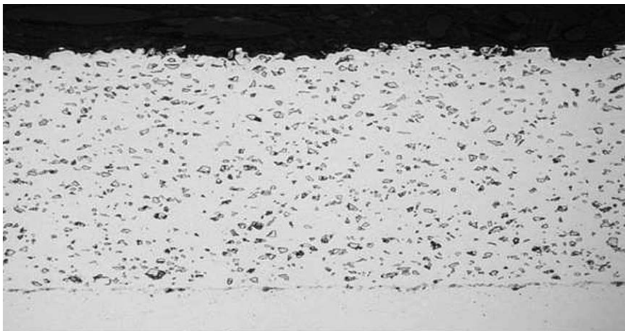
Figure 1: TriCom is a composite coating consisting of a cobalt matrix with chromium-carbide reinforcing phase.
