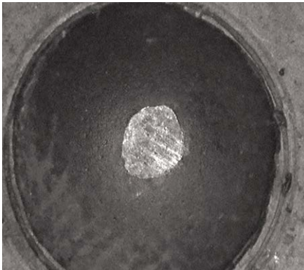
Figure 3: TriCom exhibited excellent wear resistance at 1150°F, surviving 4.9 miles of sliding wear on a 10mm ball. Wear scar diameter is 0.022 inches.
